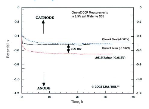
These studies indicate no detrimental effects of connecting ChromX® and carbon steel reinforcement together.
